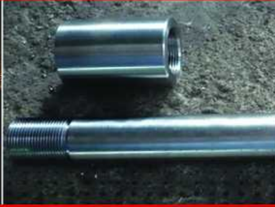
METAL SPRAY COATING (SHAFT & HOUSING BEARING)
